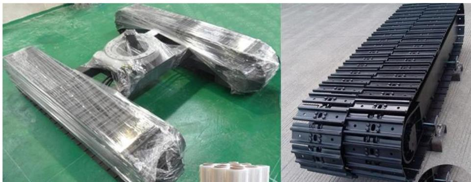
1.Wrap the undercarriage with wrapping film
